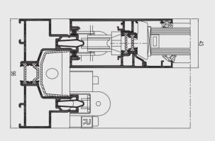
The CP 96 sliding and lift & slide elements are the perfect answer to the increasing demand for safety and durability at a fair price. They are combined with strong technical performance to make up a very reliable system. The CP 96-AP variant is available in slide and lift & slide version and offers an enhanced burglary resistance variant.
